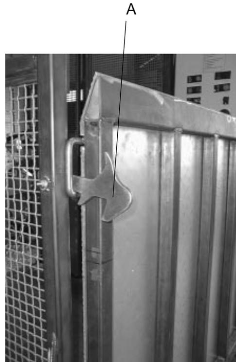
Fig.7-5 Locking sliding gate
