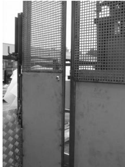
Fig.6-7 Assembly platform door
