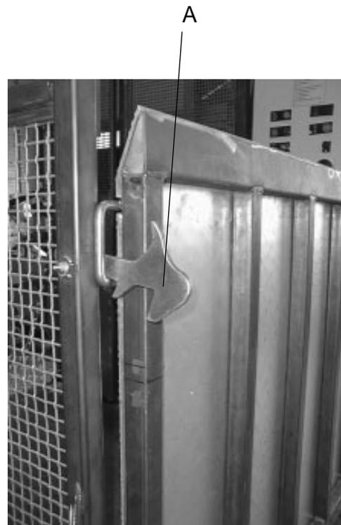
Fig.7-5 Locking sliding gate
