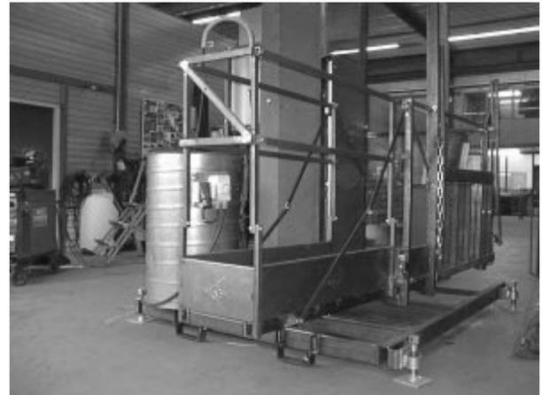
*Fig.8-1 Assembly platform*
